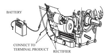
Use 12V and more than 18A.H battery, connect its positive lead to start relay terminal while connect its negative lead to engine mounting screw, base screw or other grounding point with the engine. (See Fig. 2)
